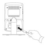
2. Press the WPS button on your wireless device then press the WPS button on the camera.
